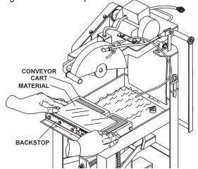
Figure 25. Material Placement
